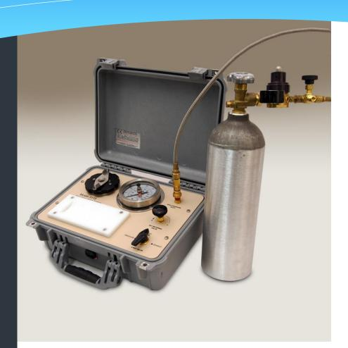
SAPS II PLANT WATER STATUS CONSOLE, 25 Bar Gauge, G4 Specimen Holder in carry case, 22 c/f tank (empty) included:
