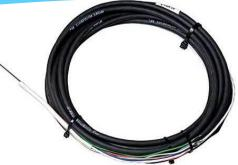
The ST-150 is a 1/8 inch, Class A PRT with an IP67 rating. White heat shrink is used on the cable behind the PRT to minimize heat transfer to the sensor. PRT sheath dimensions are 3.18 mm diameter and 57.15 mm length, minimizing thermal mass.
